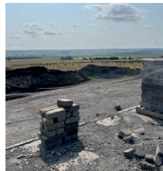
Fly ash beneficiated from coal waste used to produce green cement, bricks, pavers, barricades
